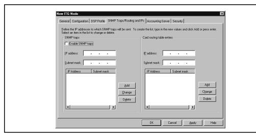
Check the Enable SNMP traps check box to enable sending of SNMP traps to the SNMP managers that appear in the list. You must enter at least one SNMP trap address if you check this option. The SNMP trap addresses determine where event and alarm messages are sent.
